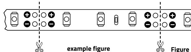
Separate the VARDIFLEX LED strip at the marked position. For a tightly assembled LED strip a micro side cutter or an optional cutter required.
